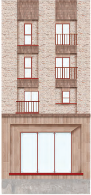
Above: Brick, GFRC, and terracotta form a resilient, low-maintenance envelope with warmth and texture. The high-performance wall assembly achieves a U-value of 0.14 W/m 2 K, reducing heat loss, enhancing comfort, and maximizing daylight."
