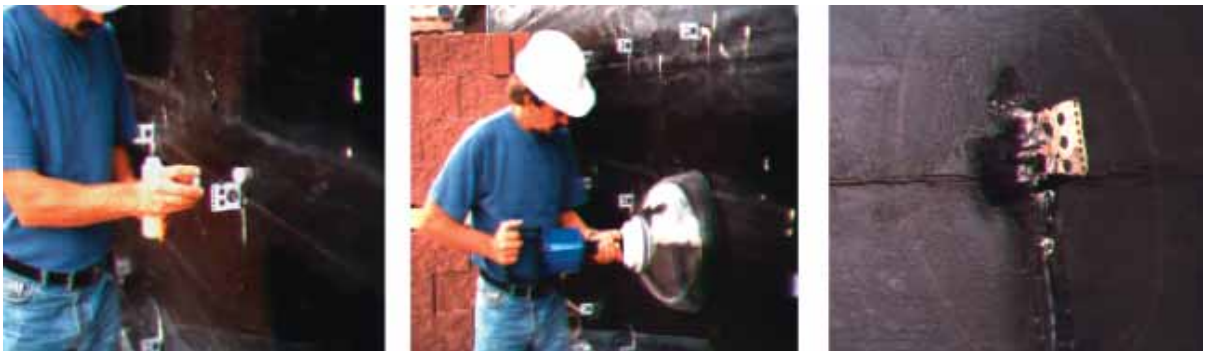
Figure 14: ASTM E 4.2.7 test being performed on a masonry tie. Photo 1, leak detection solution is applied around the penetration. Photo 2, Leak Detector unit is placed over the detail and activated, creating a pressure differential within the clear test chamber. Photo 3, bubbles indicate the presence and location of a leak.
