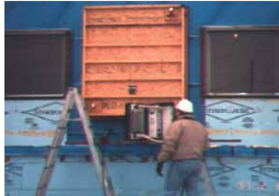
Figure 12: Conducting an ASTM E 783 test.
