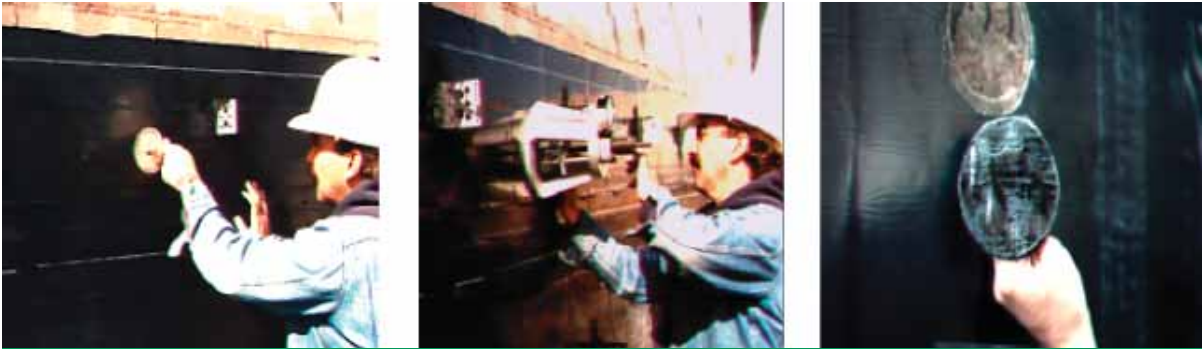
Figure 13: ASTM D 4541 membrane-substrate adhesion test. Photo 1, installer makes a cut in the membrane by tracing around the adhesion pad. Photo 2, bond adhesion tester is used to place a load against the membrane. Photo 3, membrane becomes detached from the wall as a result of the load placed against it.
